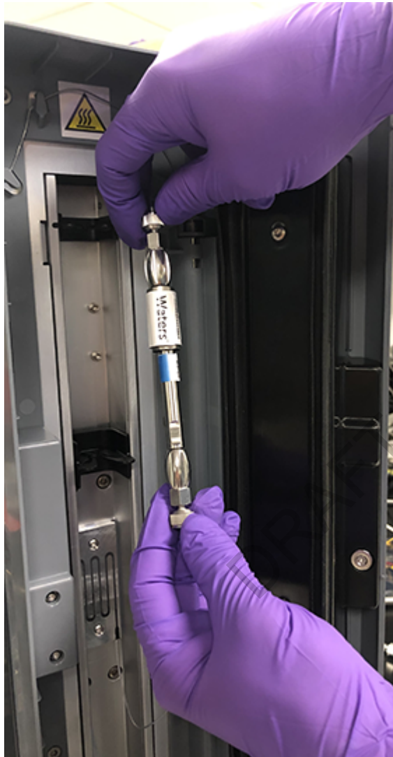
Figure 4–4: Installing the replacement column
