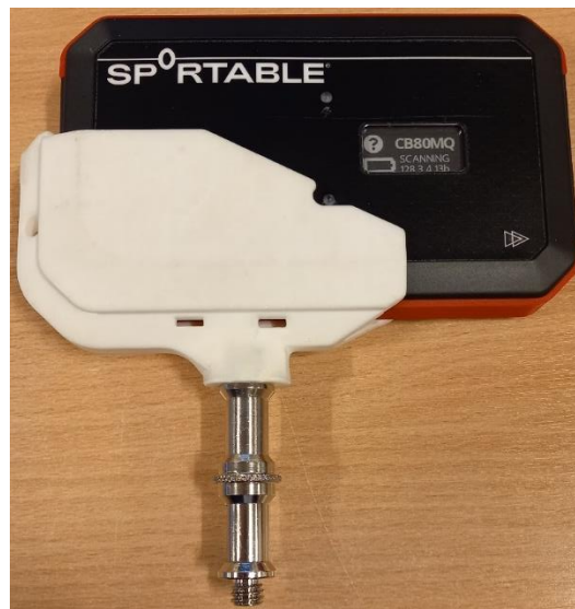
Lynx device in bracket using bottom mounting thread
