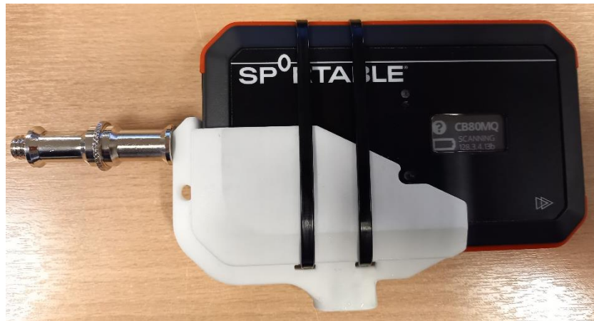
Lynx device in bracket using side mounting thread
