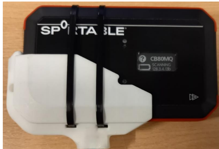
Lynx device secured into bracket using tie wraps (front view)
