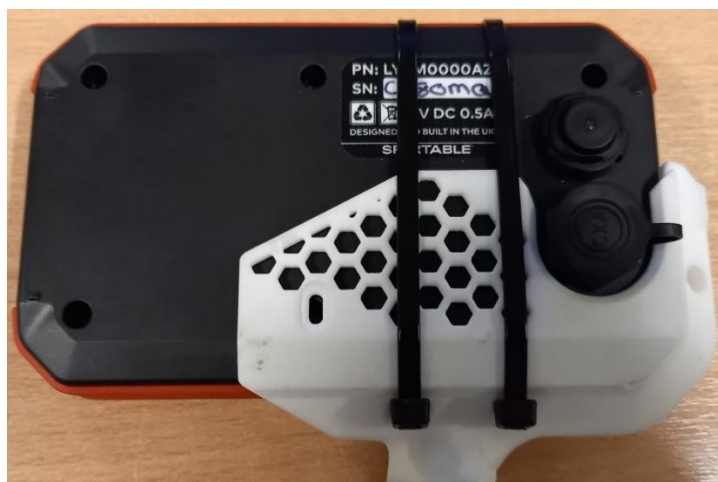
Lynx device secured into bracket using tie wraps (rear view)
