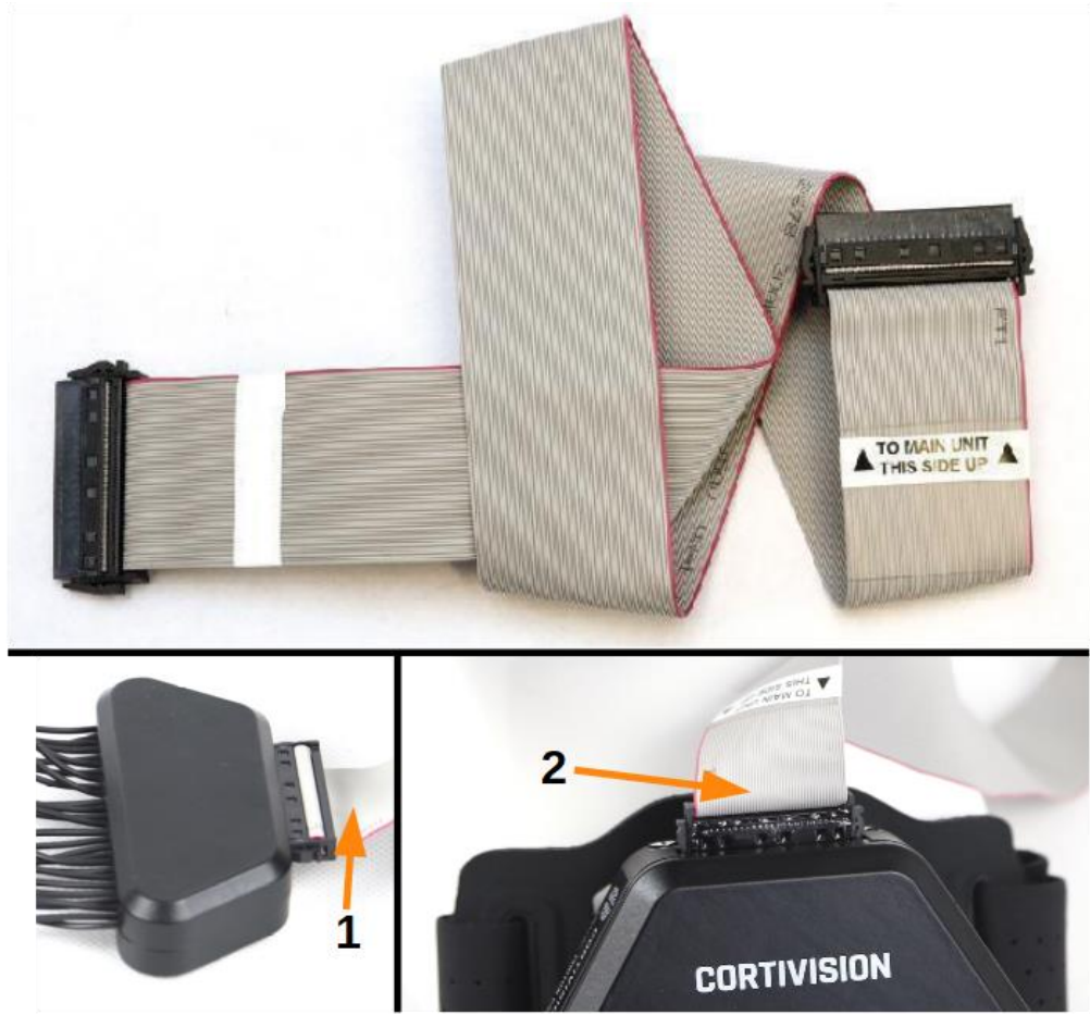
Fig. 5. Flat cable: 1. Plug to be connected to the socket in the distributor, 2. Plug to be connected to the socket on the amplifier.
