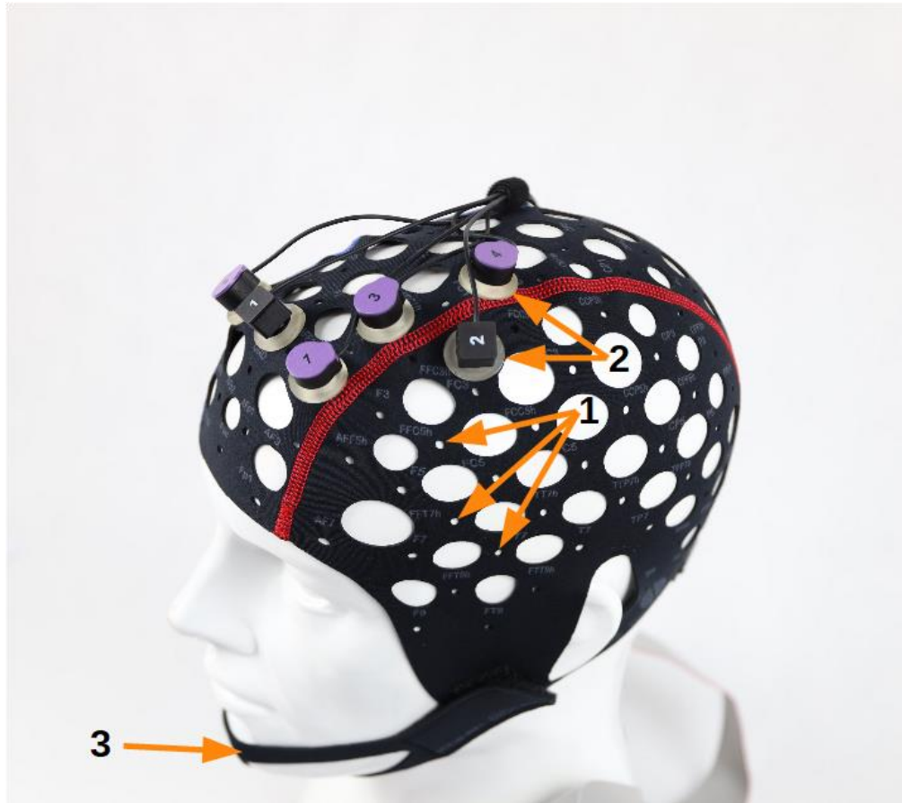
Fig. 3. Cap: 1. Holes for mounting optodes, 2. Optode mounts, 3. Chinstrap.
