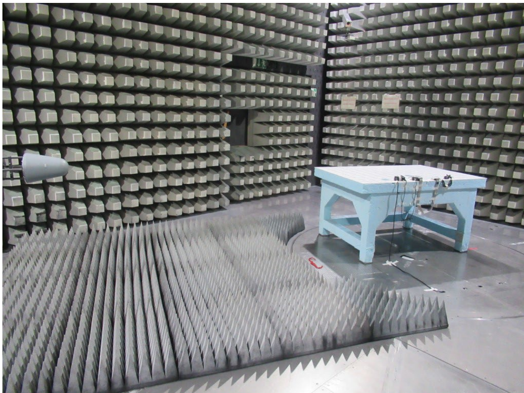
Photo 8: Radiated Test Setup from 1 GHz to 15 GHz
