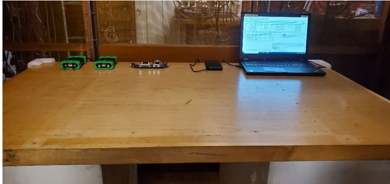
Figure 7: Conducted Emissions Test Setup Photograph(s).
