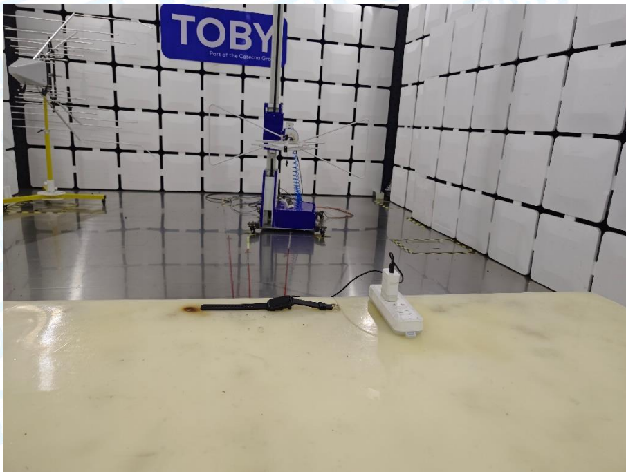
Photo of Setup for Radiated Emission (30MHz~1GHz)
