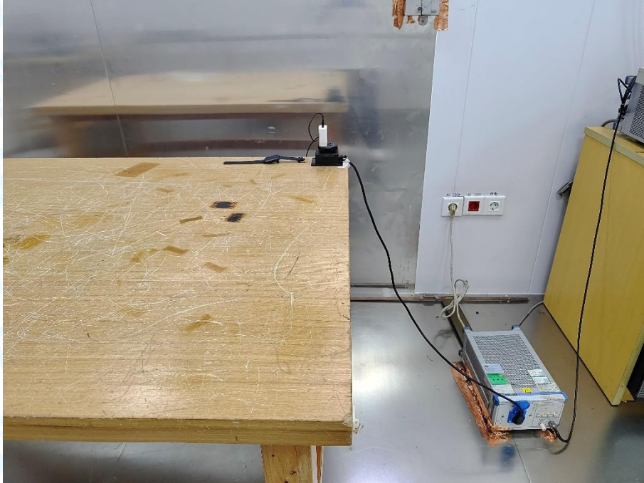
Photo of Setup for Radiated Emission (30MHz~1GHz)
