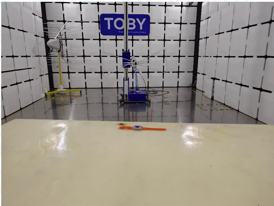
Photo of Setup for Radiated Emission (30MHz~1GHz)
