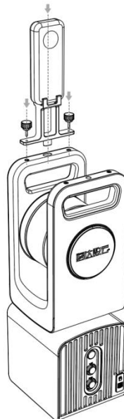
Figure 3-2.3 Installation diagram of HD TLS360 system camera
