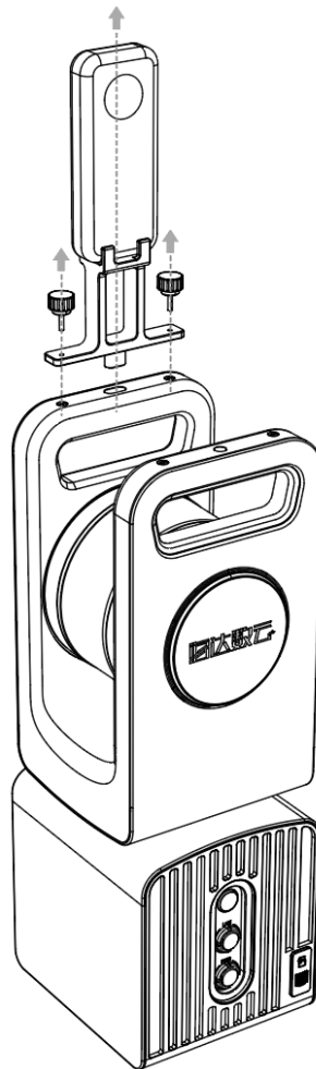
Figure 3-2.4 Disassembly diagram of HD TLS360 system camera
