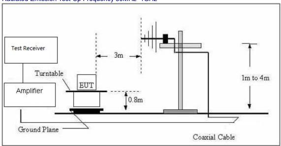
(C) Radiated Emission Test-Up Frequency Above 1GHz
