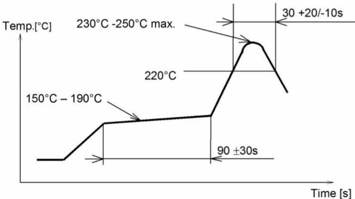
Maximum number of cycles for re-flow is 2. No opposite side re-flow is allowed due to module weight.
