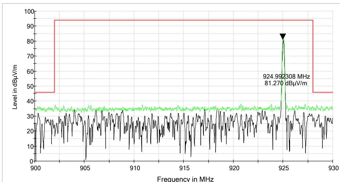
**Band Edge and Field Strength of the Fundamentals**
