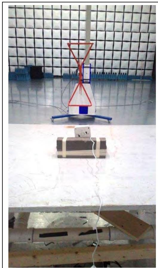
**Radiated Spurious Emissions Greater than 1 GHz**
