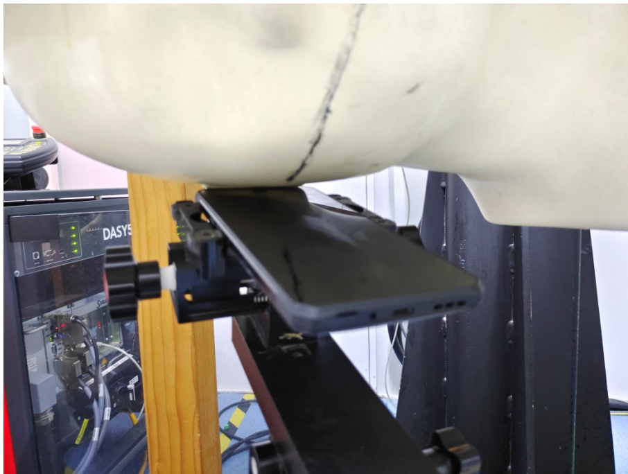
Head Right Tilt Setup Photo (0mm)
