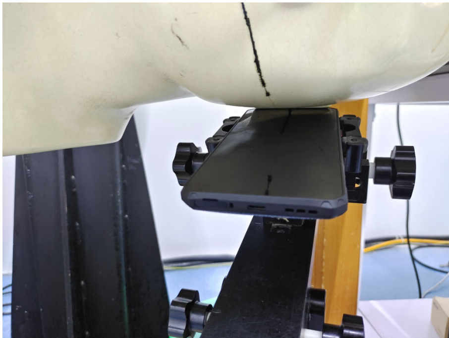
Head Left Tilt Setup Photo (0mm)
