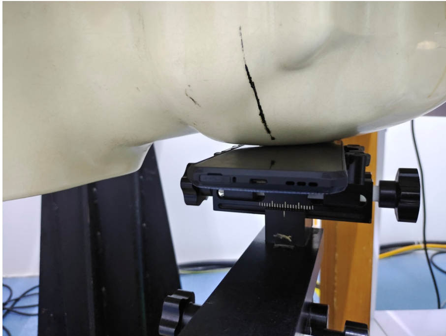
Head Left Tilt Setup Photo (0mm)
