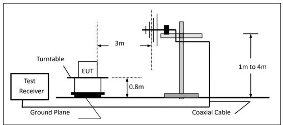
(c) For radiated emissions above 1000MHz
