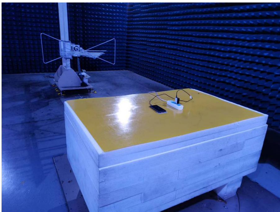
Photo of Radiated Emission Measurement (30MHz-1GHz)
