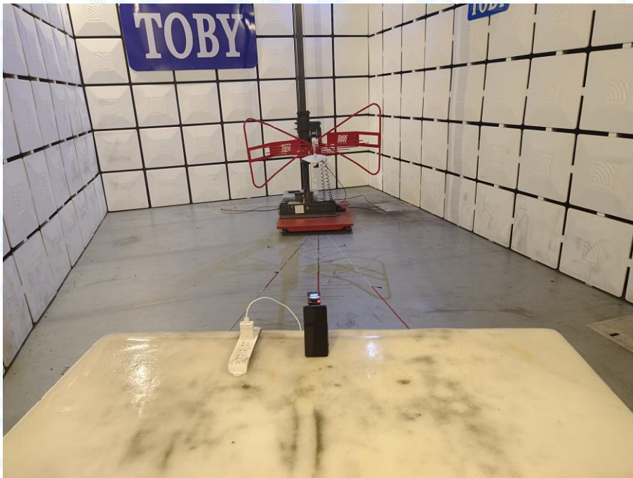
Photo of Setup for Radiated Emission (9KHz-30MHz)
