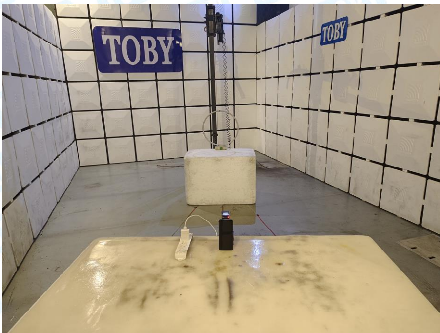
Photo of Setup for Radiated Emission (9KHz-30MHz)
