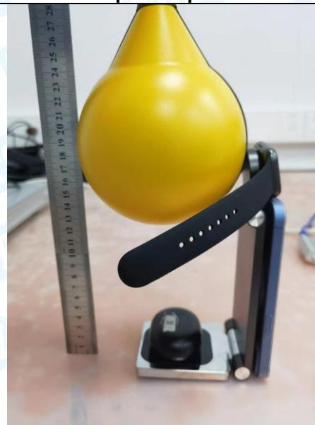
**H-Field Strength-15cm****Test Position A - Exposure photo from side edge surface-Rear**
