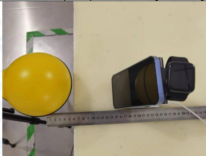
**H-Field Strength- 15 cm (Watch Ant3)****Test Position E - Exposure photo from top surface**
