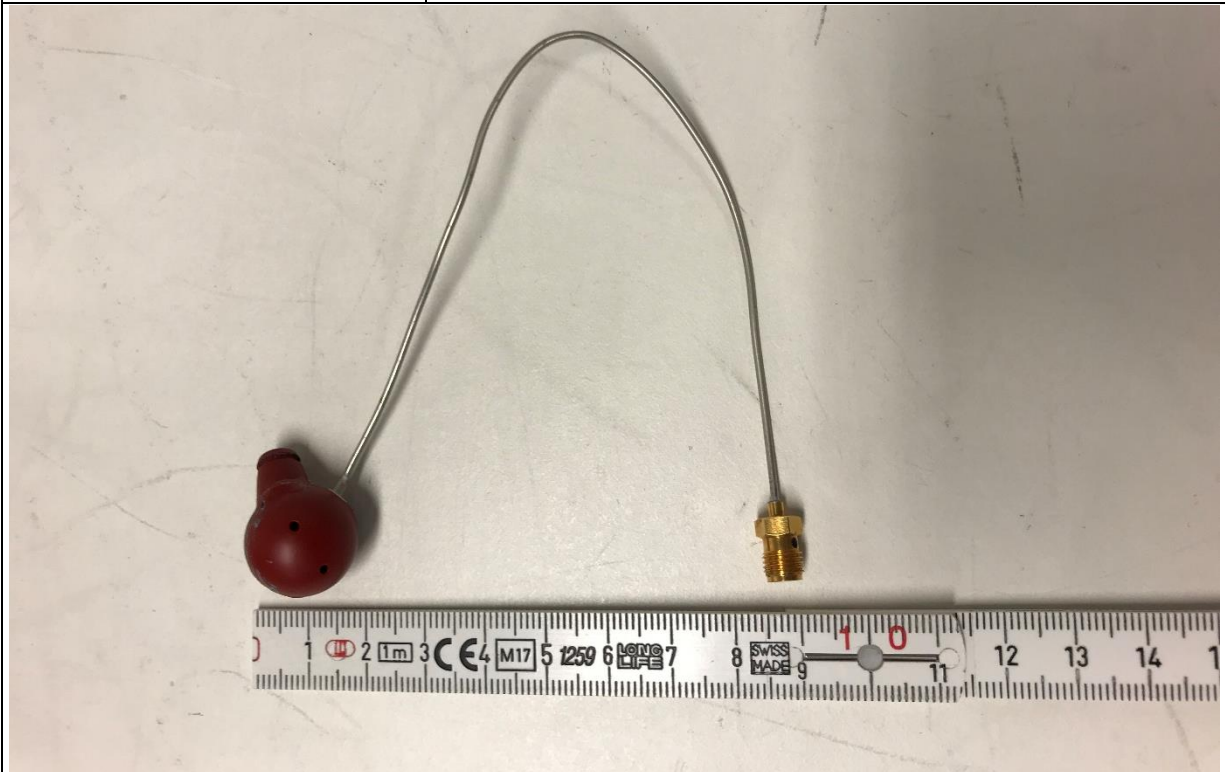
Photo 1.1.2 .....: Test item 2 PCB with BLE antenna replaced with SMA connector
