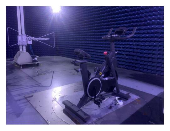
Photo of Radiated Emission Measurement Above 1GHz
