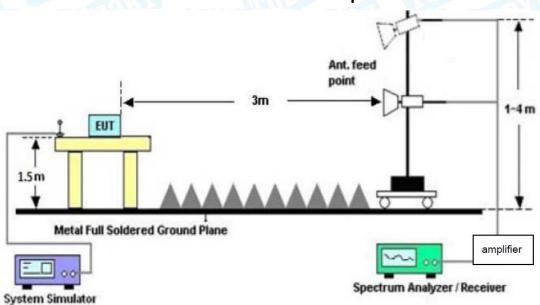
**Above 1GHz Test Setup**
