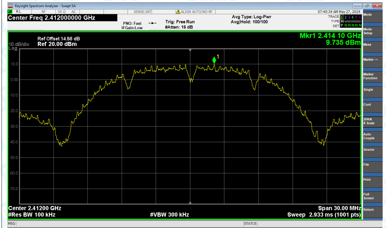
Tx. Spurious NVNT b 2412MHz Ant1 Emission
