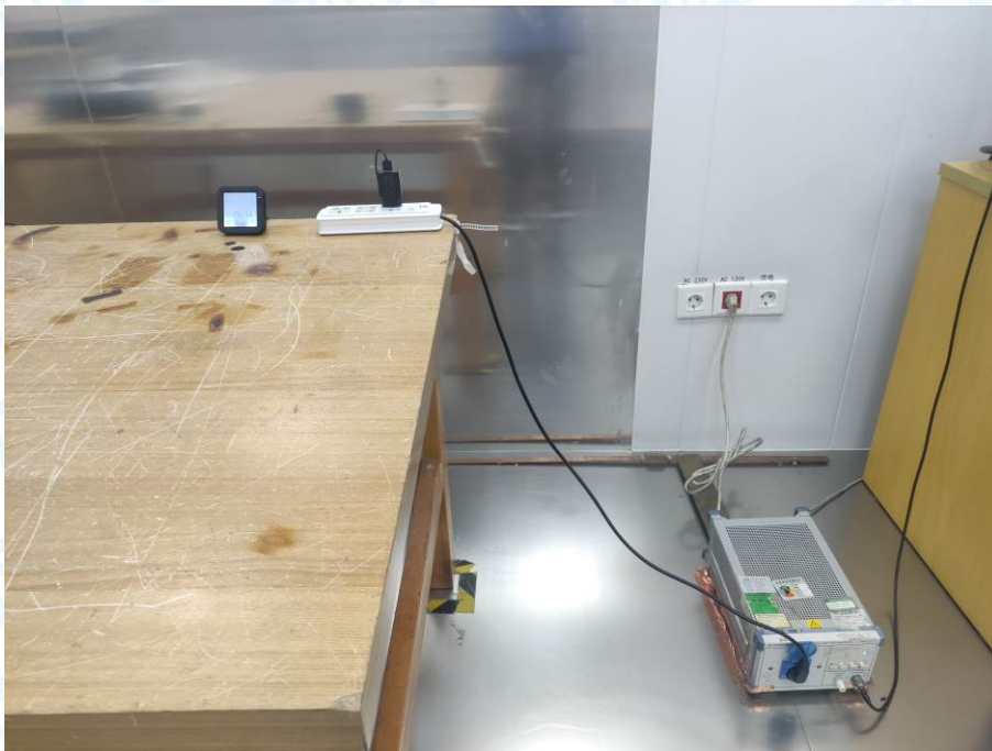
Photo of Setup for Conducted Emission
