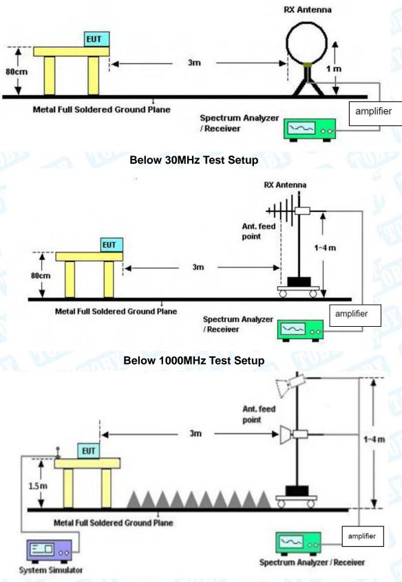
Above 1GHz Test Setup
