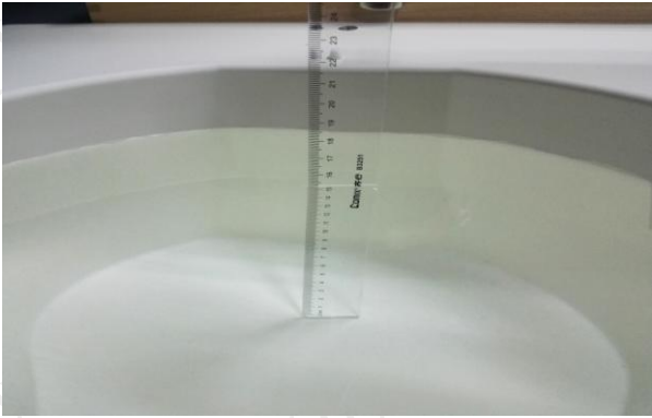
The Body Liquid of 2450MHz (15.3cm)
