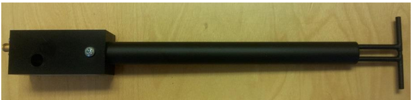
Figure 1 – MVG COMOSAR Validation Dipole
