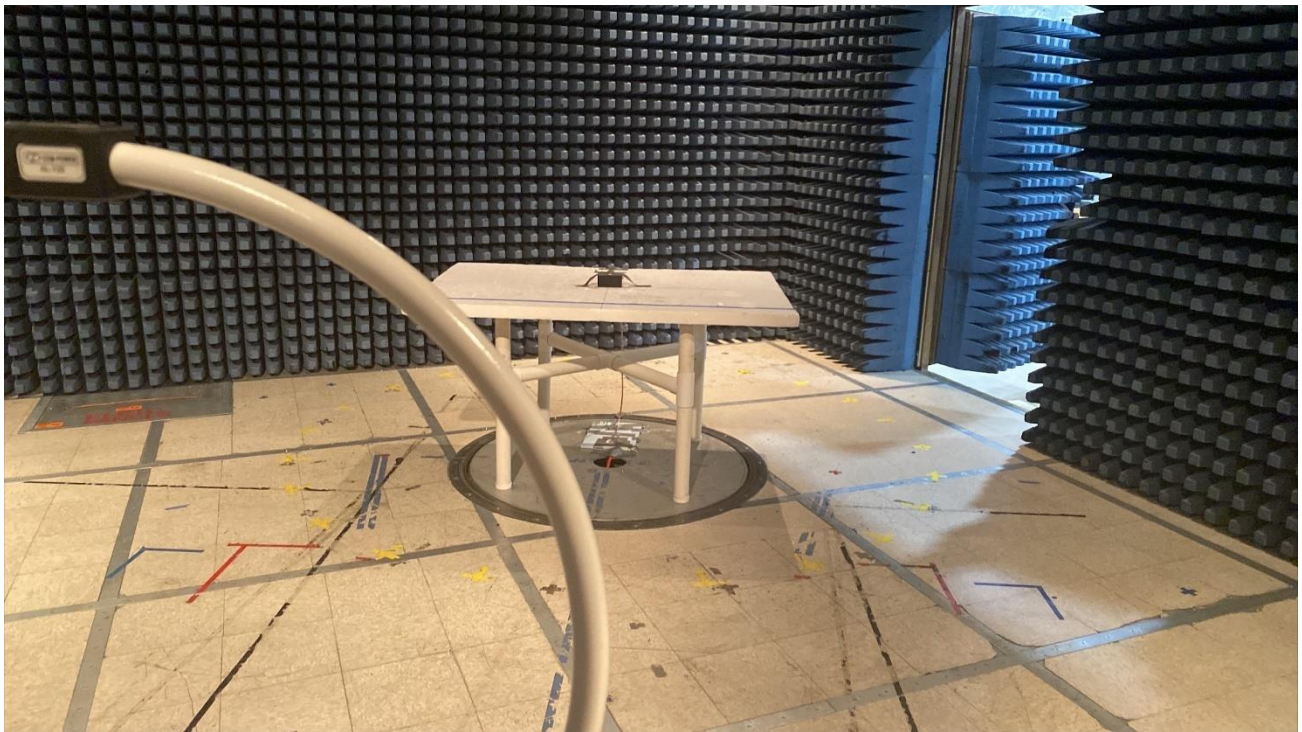
Figure B-2 - Radiated Emissions Measurements Below 30MHz
