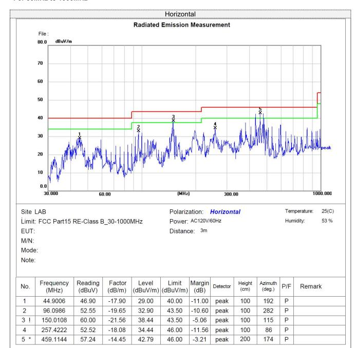
Note:1).Level ( $dB\mu V/m$ )= Reading ( $dB\mu V$ )+ Factor (dB/m)
