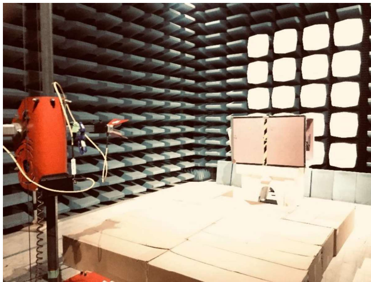
Figure 31: Radiated Emissions above 1GHz performed at the 3m SAC
