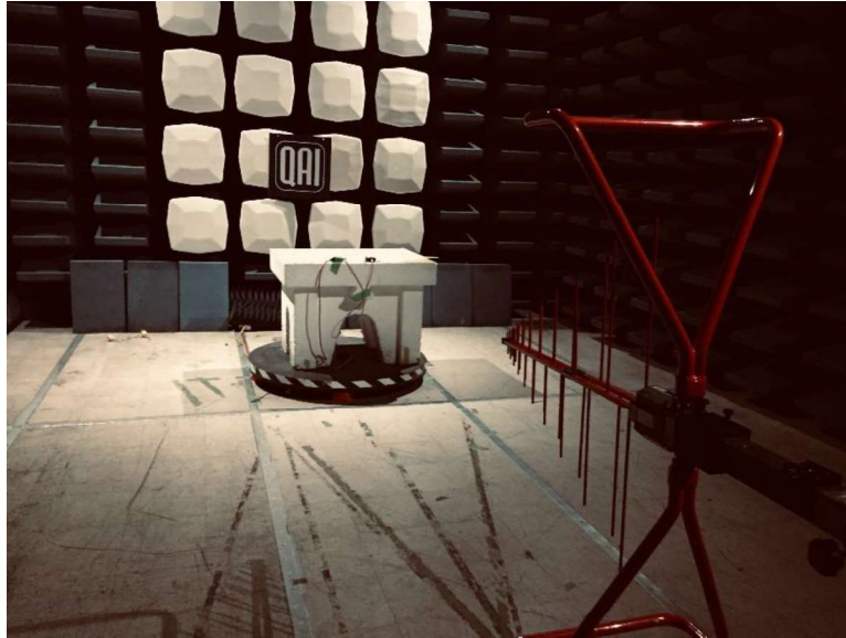
Figure 30: Radiated Emissions performed at the 3m SAC, 30MHz – 1GHz Charging Mode
