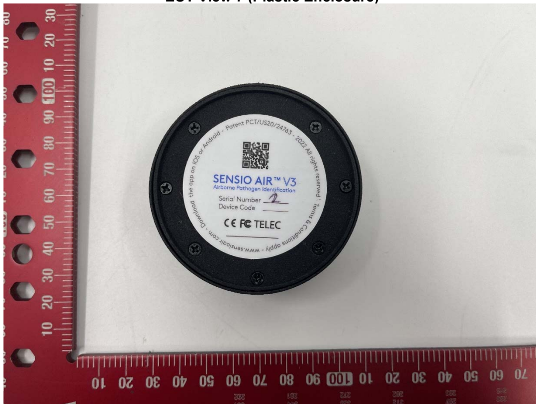
EUT View 8 (Plastic Enclosure)
