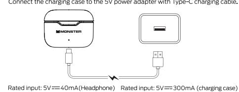
Rated input: 5V=40mA(Headphone) Rated input: 5V=300mA (charging case)
