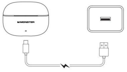
Rated input: 5V === 40mA(Headphone) Rated input: 5V === 200mA (charging case)
