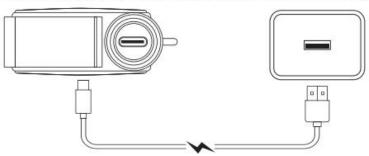
Rated input: 5V== 30mA(Headphone) Rated input: 5V== 200mA (Charging case) Tips: When the ice blue indicator flashes while closing the cover, please charge in time.
