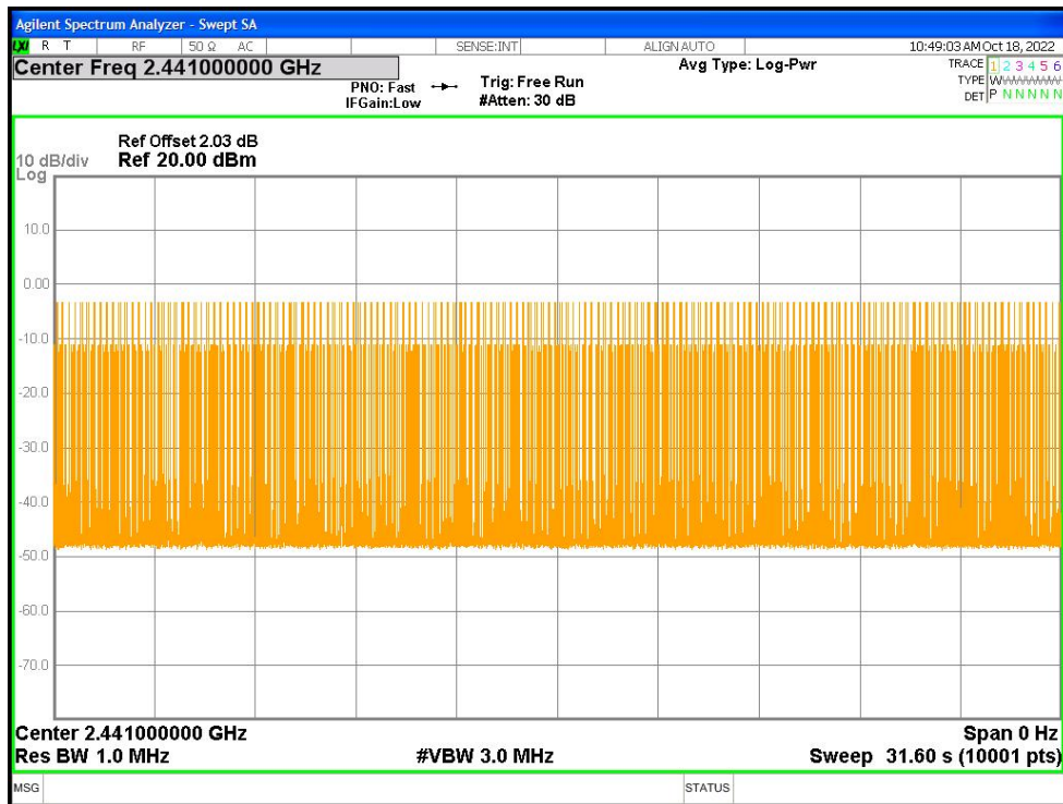
Dwell NVNT 1-DH3 2441MHz Ant1 One Burst
