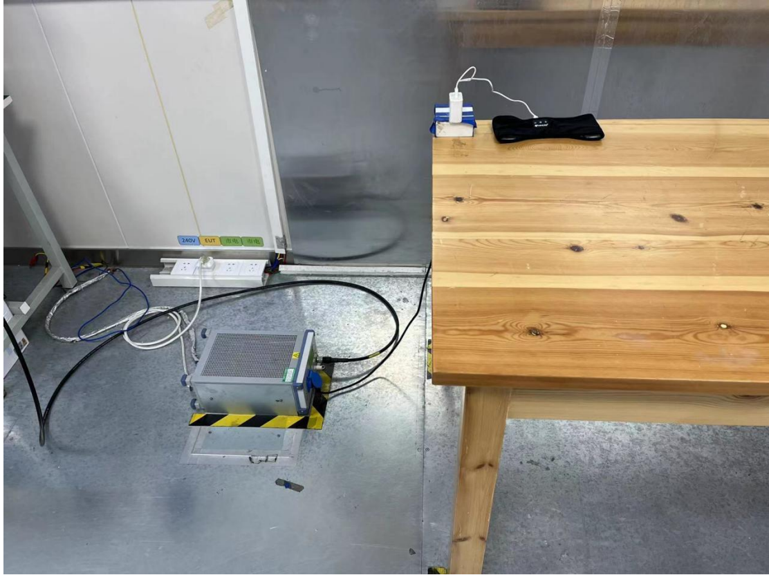
Conducted emission test setup
