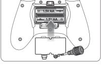
c) Cover up the battery cover, and tighten the screws.
