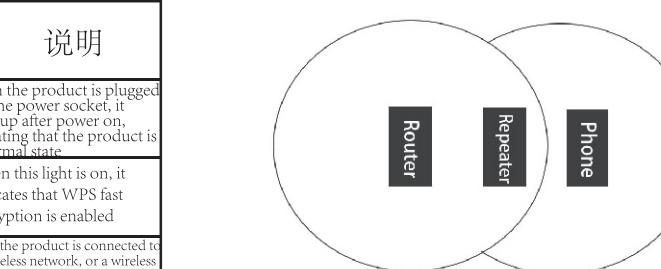
As a WiFi signal extender, repeater can expand your WiFi signal without using any cables, reducing the trouble of wiring, but can't optimize the speed of WiFi.
