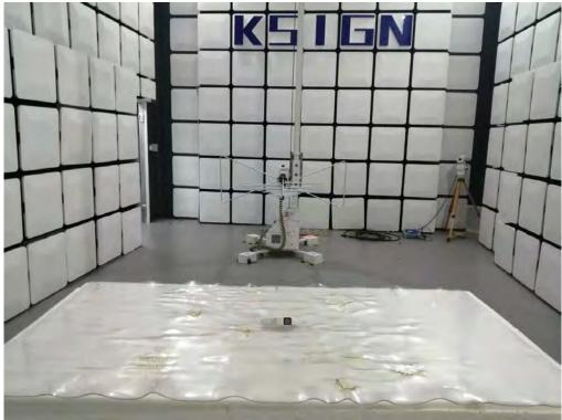
Radiated Measurement (Above 1GHz)
