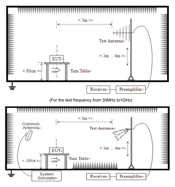
(For the test frequency above 1GHz)
