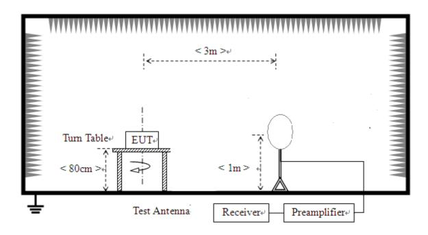
For radiated emissions from 30MHz to 1GHz
