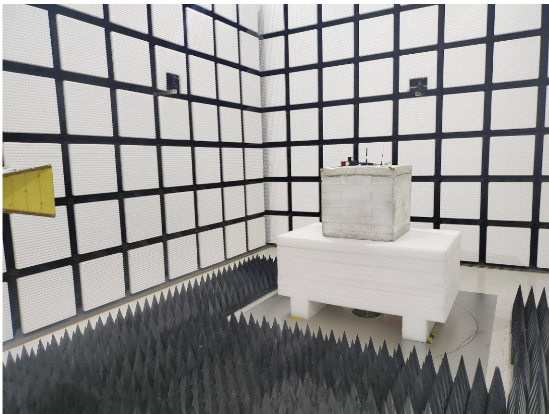
Radiated Emission Above 1GHz View
