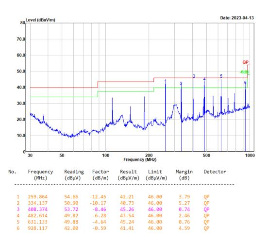
Test Mode: Monitoring&Charging Polarization: vertical
