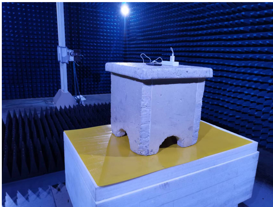
Photo of Radiated Emission Measurement (Above 1G)
