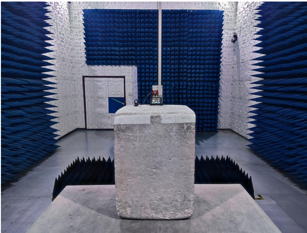
RADIATED EMISSION TEST SETUP ABOVE 1GHz
