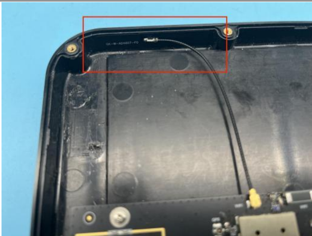
Schematic diagram of the installation position of the built-in WiFi antenna
