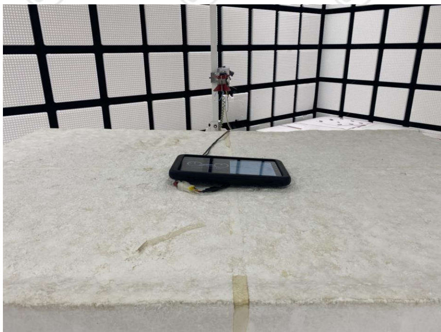
Radiated spurious emission Test Setup-2(Above 1GHz)
