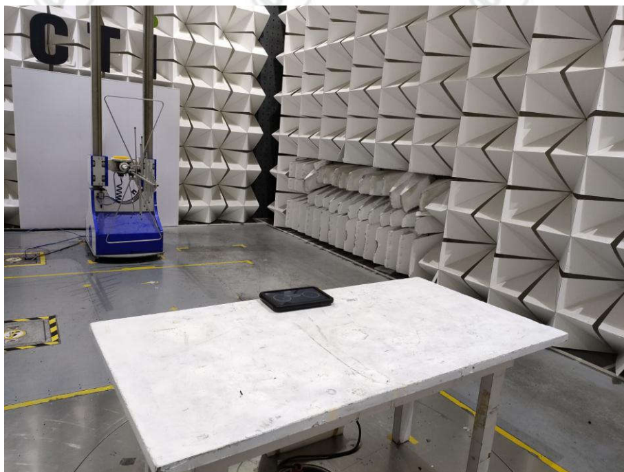
Radiated spurious emission Test Setup-1(Below 1GHz)
