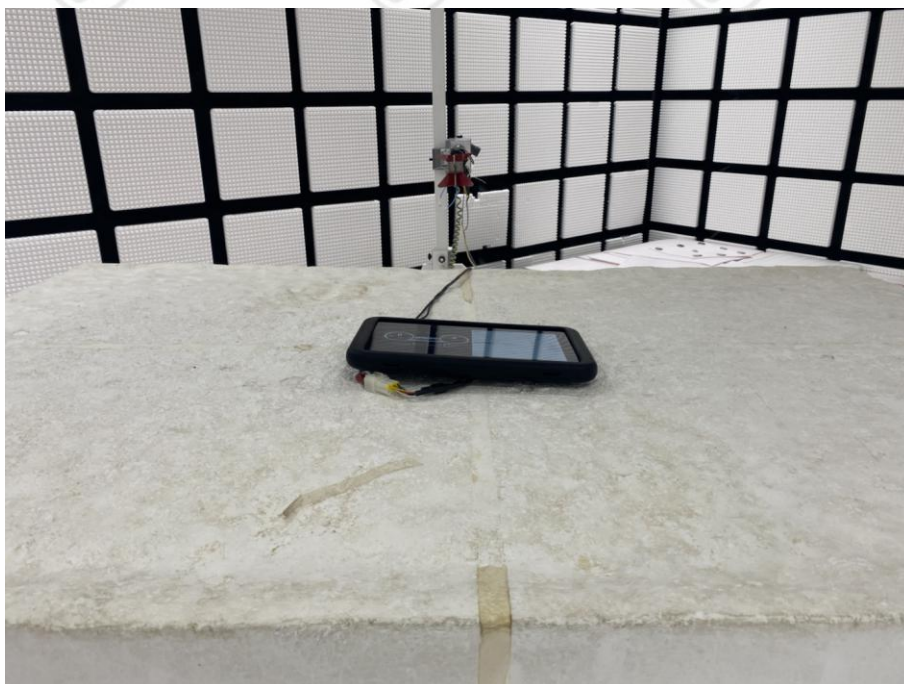
Radiated spurious emission Test Setup-2(Above 1GHz)
