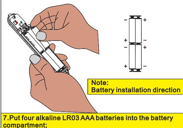
7. Put four alkaline LR03 AAA batteries into the battery compartment;
