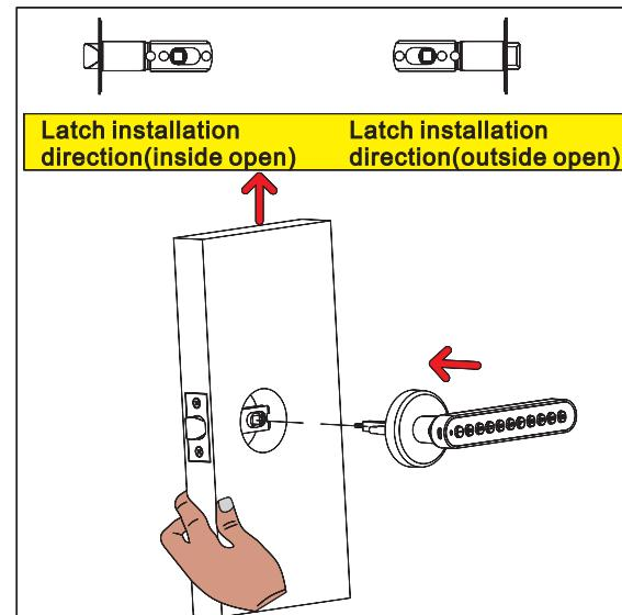
8. Align the front handle with the door hole and pass through the lock hole;
