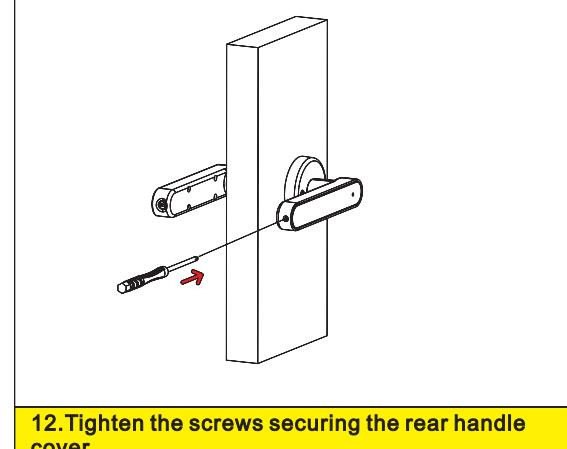
12. Tighten the screws securing the rear handle cover.
