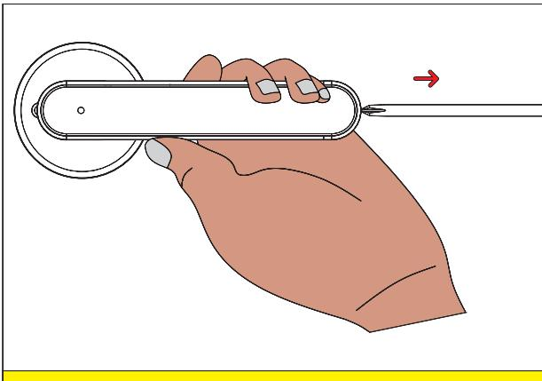
6. Use a screwdriver to remove the screws on the rear handle cover.
