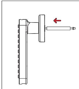
4. Put the front handle wire through the middle of the 100 square cylinder;
