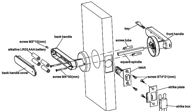
**TIPS:** 1. Install the spindle into the latch, and get the cables through the middle of spindle.
