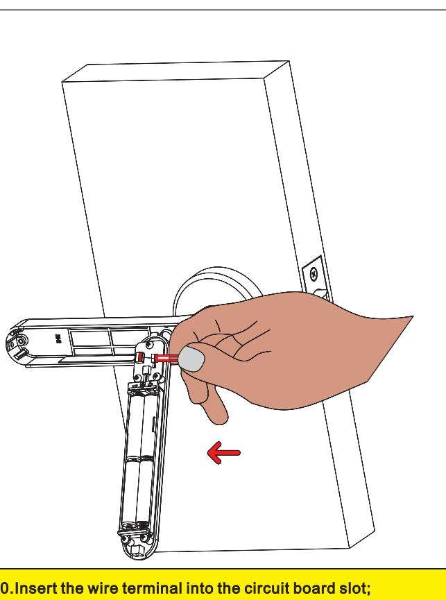
10. Insert the wire terminal into the circuit board slot;
