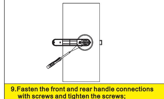
9. Fasten the front and rear handle connections with screws and tighten the screws;
