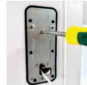
Tighten the screws after keeping the built-in board and the front panel vertical
