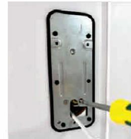
Align the holes of the built-in board and fix them with flat head screws
