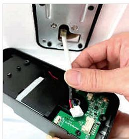
Insert the cable into the connector
