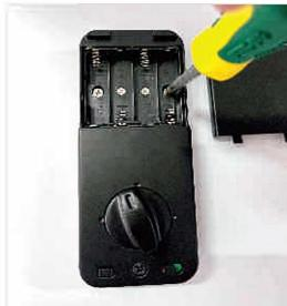
Remove the built-in screws on the rear panel and take off the built-in board
