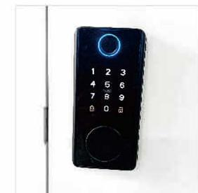
After installing the battery, please test whether the left and right door opening positions are correct. If the switch direction is opposite, please wake up the screen and input "666888#", and hear a long "beep", which means that the direction switch is not successful.
