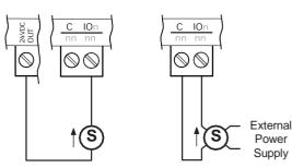
Note: The 24VDC OUT terminal can source up to 75 mA.
