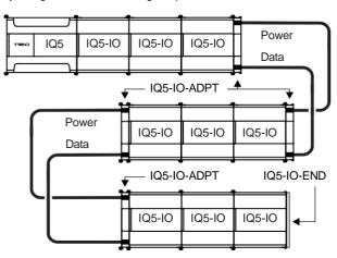
Note: The IQ5-IO-ADPT wiring adapter includes a self-resetting fuse and transient voltage suppression that protects the I/O bus from over-current and over-voltage conditions caused by electrical transients or incorrect wiring. No protection is provided against accidental connection of mains voltages.
