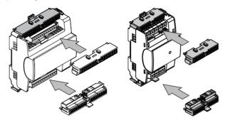
The AUX-TRM-16 has 16 push-fit terminals, configured as two common groups of 8 and suitable for all 105mm wide modules. The AUX-TRM-10 has 10 push-fit terminals, configured as two common groups of 5 and suitable for all 70mm wide modules. Both blocks can carry a maximum load of 12 A.
