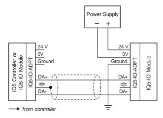
Important: The 24 Vdc connection from the previous module must not be made. The 0 V connection must be made when an external supply is used and the 0 V line must be continuous for the entire length of the I/O bus.
