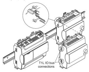
Note: Modules can easily be removed without disturbing adjacent modules.
