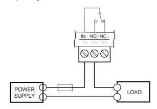
Ensure that external circuits are suitably protected against fault currents that would exceed the ratings for the switching circuits provided in this product.
