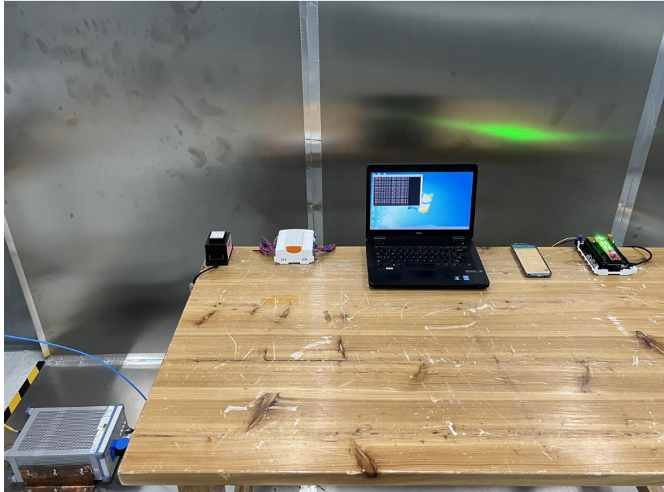
Photograph 3: Set-up photo for Conducted Emission on AC Mains
