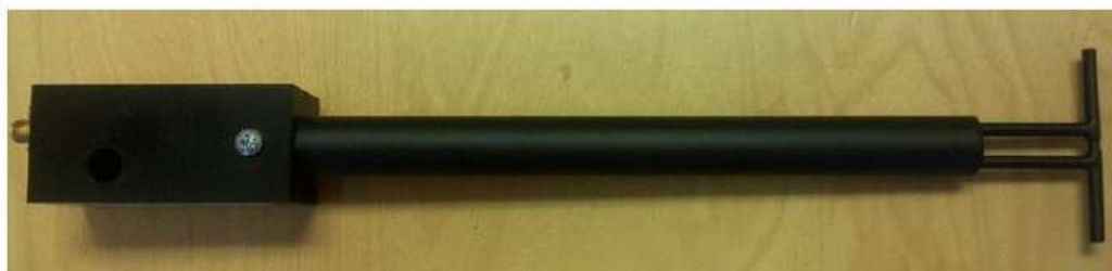
Figure 1 – MVG COMOSAR Validation Dipole
