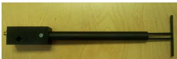
Figure 1 – MVG COMOSAR Validation Dipole
